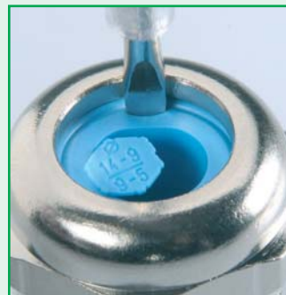
Fig. 3 With a large cable diameter—remove inlet. Insert screwdriver vertically into separating seam
