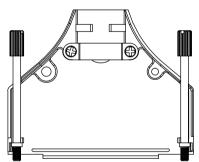
BACKSHELL MATERIAL: PLATING: JACKSCREWS: M3 HOODSCREWS: COMPRESSION INSERT: METAL CLAMP: CLAMP SCREWS: OPERATING TEMP: DIE—CAST ZINC ALLOY NICKEL STEEL:ZN PLATED STEEL:ZN PLATED ABS,UL RECOGNIZED STEEL:ZN PLATED STEEL:ZN PLATED -40°C TO+120°C
