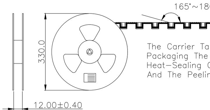
The Carrier Tape Is Heat-Sealed Packaging The Peeling Angle Of The Heat-Sealing Cover Tape Is 165°~180° And The Peeling Force Is 30~120g.
