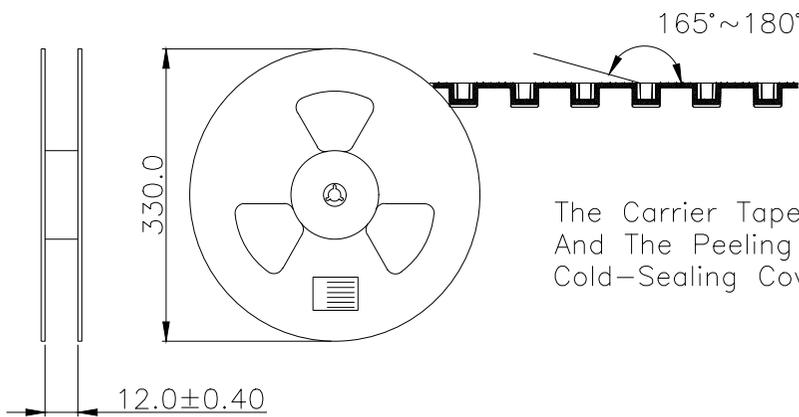
The Carrier Tape Is Cold-Sealed And The Peeling Angle Of The Cold-Sealing Cover Tape Is 165°~180°.
