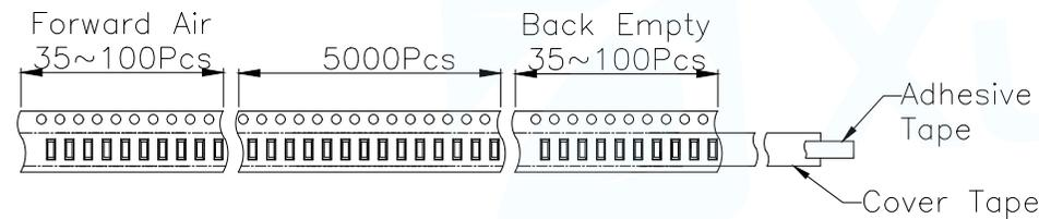
Customer To Use Direction Pull Out Direction (出料方向)
