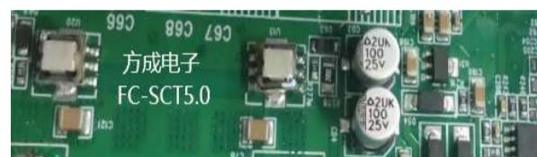
It is used as DC current transformer for various electronic device detection
