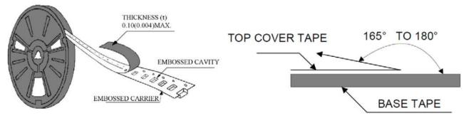
The force for peeling off cover tape is 10 to 70 grams in the arrow direction.
