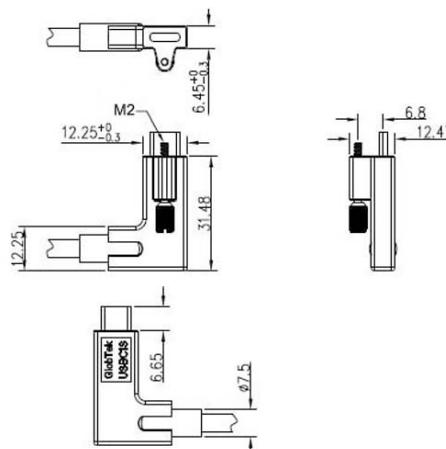
Mates with GlobTek USB Type C cables with 2 screws.
