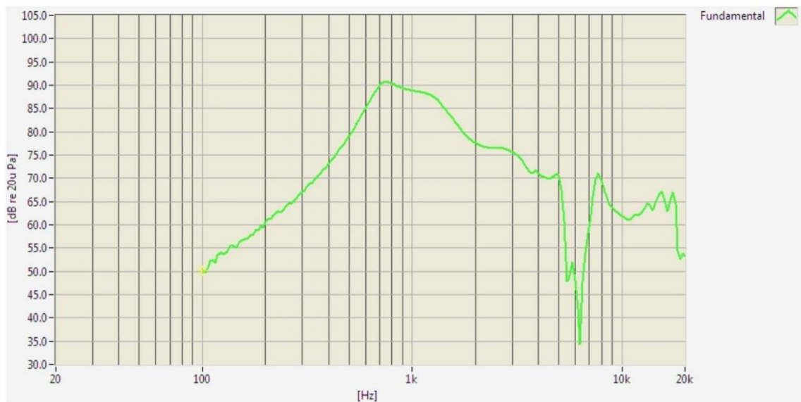
Fig.2 Typical frequency response curve (speaker mode)
