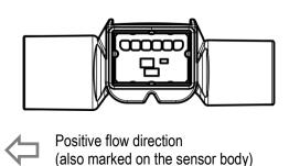
Positive flow direction is from the male 15 mm cone to the female 15 mm medical cone, so that inspiratory flows are positive and expiratory flows negative.
