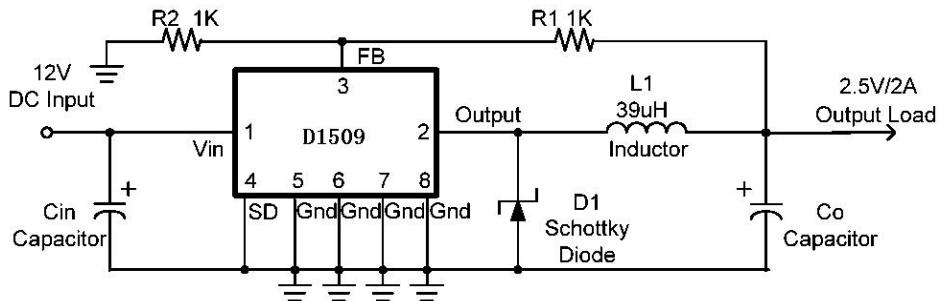
$$V_{out} = V_{FB} \times \left(1 + \frac{R_1}{R_2}\right)$$
