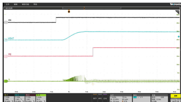
Figure 8-8. Start-Up Relative to EN Rising, Iout = 0A, OOA Mode
