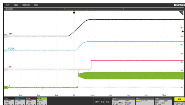
Figure 8-10. Start-Up Relative to Vin Rising, Iout = 7A
