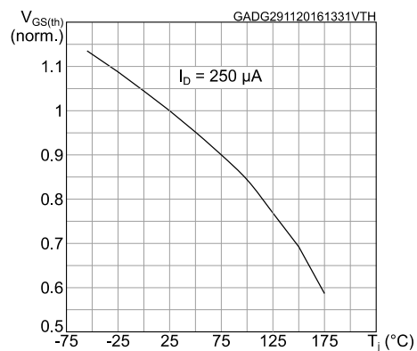
Figure 9: Normalized gate threshold voltage vs temperature
