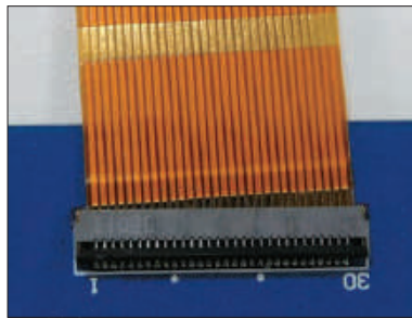
✗ Skewed FPC Insertion
