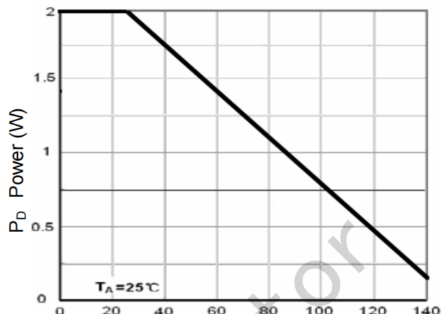
T_J -Junction Temperature(°C) Figure 9 Power Dissipation
