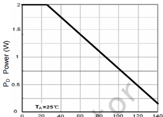
T_J -Junction Temperature(°C) Figure 9 Power Dissipation
