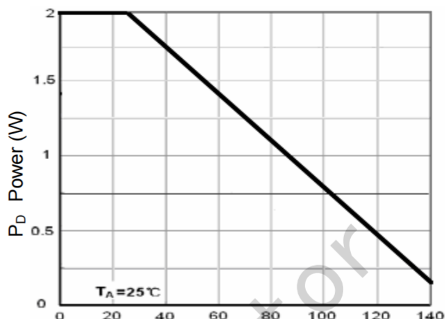
T_J -Junction Temperature(°C) Figure 9 Power Dissipation
