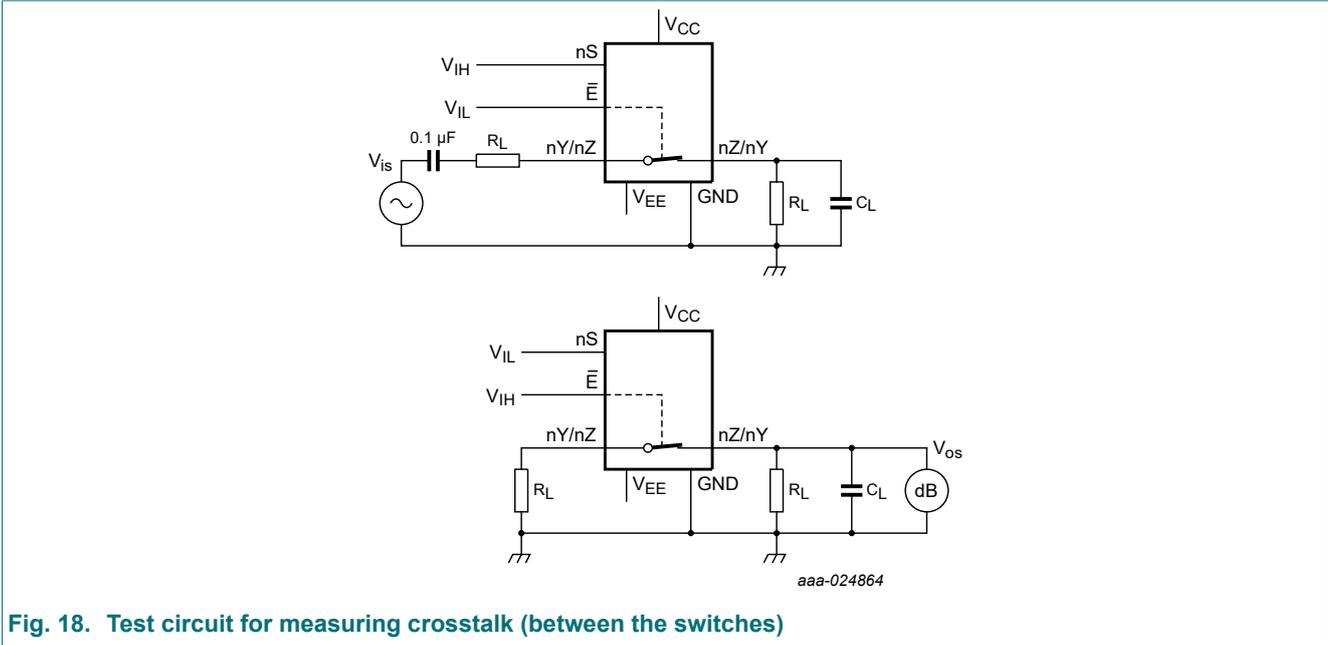
Fig. 18. Test circuit for measuring crosstalk (between the switches)
