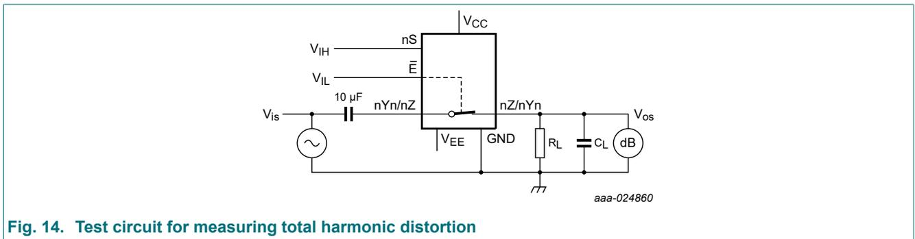
Fig. 14. Test circuit for measuring total harmonic distortion
