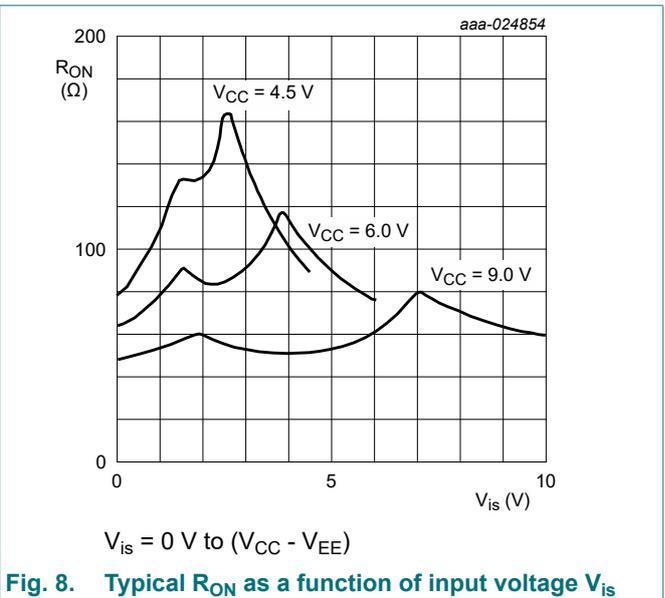
Fig. 8. Typical R<sub>ON</sub> as a function of input voltage V<sub>is</sub>
