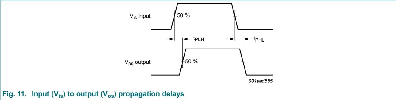
Fig. 11. Input ( $V_{is}$ ) to output ( $V_{os}$ ) propagation delays
