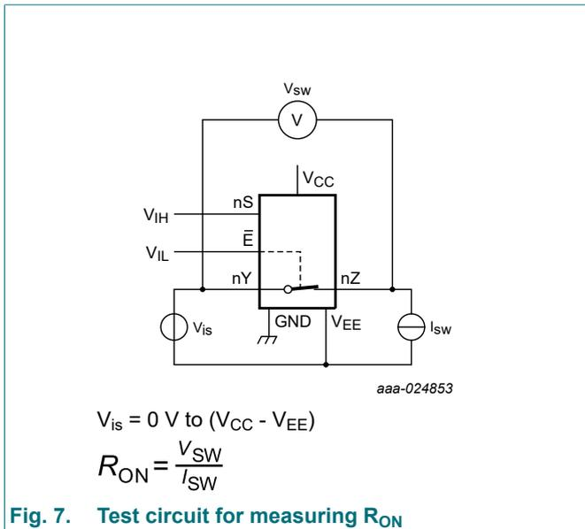
Fig. 7. Test circuit for measuring R<sub>ON</sub>
