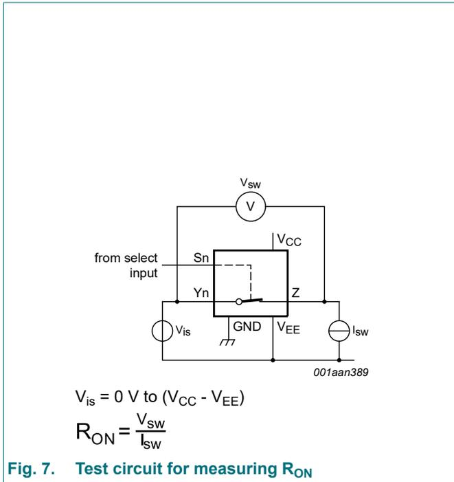
Fig. 7. Test circuit for measuring  $R_{ON}$
