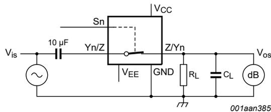
Fig. 15. Test circuit for measuring sine-wave distortion
