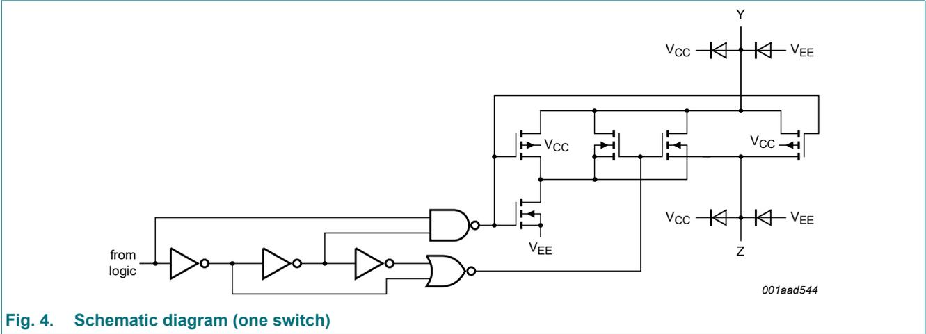
Fig. 4. Schematic diagram (one switch)
