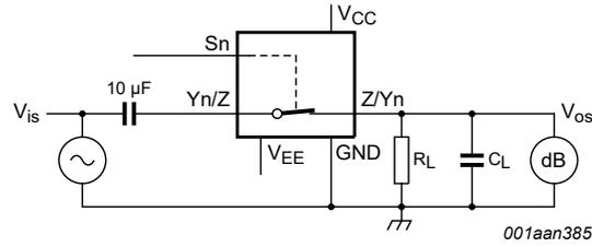
$V_{CC} = 4.5 \text{ V}$ ;  $GND = 0 \text{ V}$ ;  $V_{EE} = -4.5 \text{ V}$ ;  $R_L = 50 \Omega$ ;  $R_S = 1 \text{ k}\Omega$
