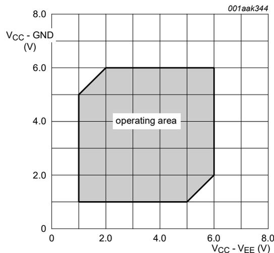
**Fig. 5. Guaranteed operating area as a function of the supply voltages**
