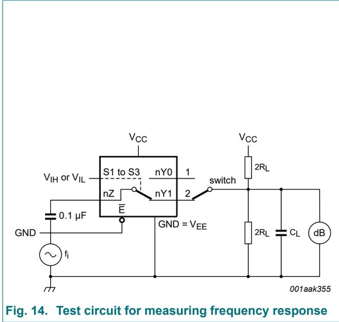
Fig. 14. Test circuit for measuring frequency response
