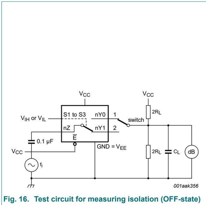
Fig. 16. Test circuit for measuring isolation (OFF-state)
