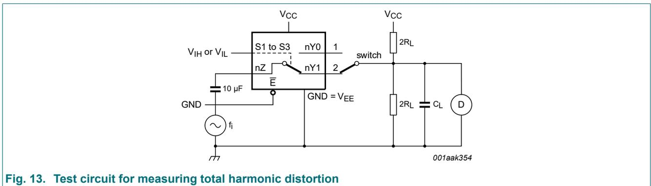
**Fig. 13. Test circuit for measuring total harmonic distortion**
