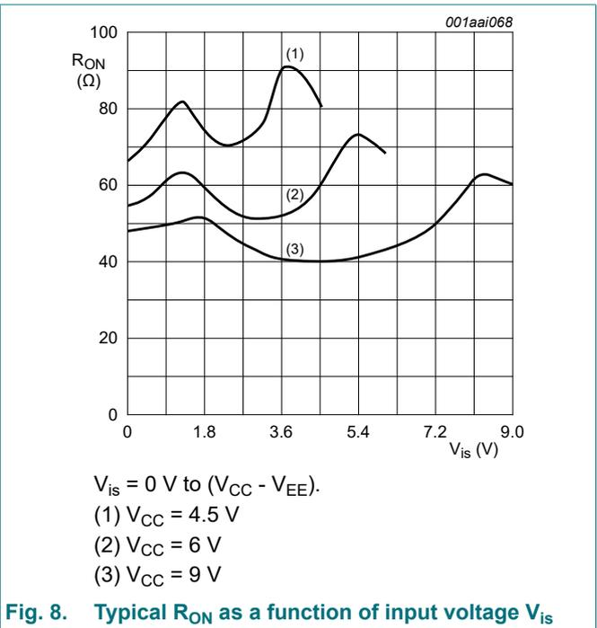
Fig. 8. Typical R<sub>ON</sub> as a function of input voltage V<sub>is</sub>
