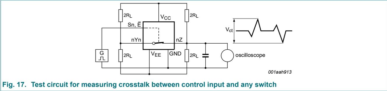
Fig. 17. Test circuit for measuring crosstalk between control input and any switch
