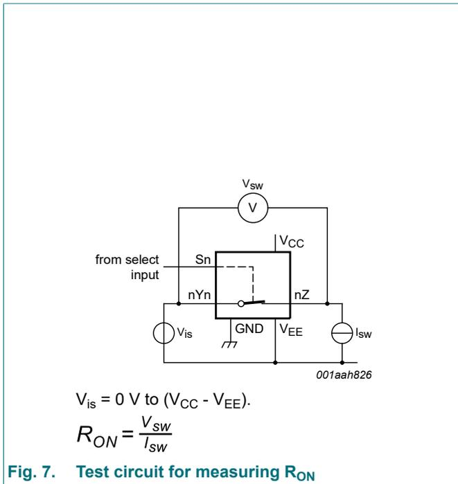
Fig. 7. Test circuit for measuring R<sub>ON</sub>
