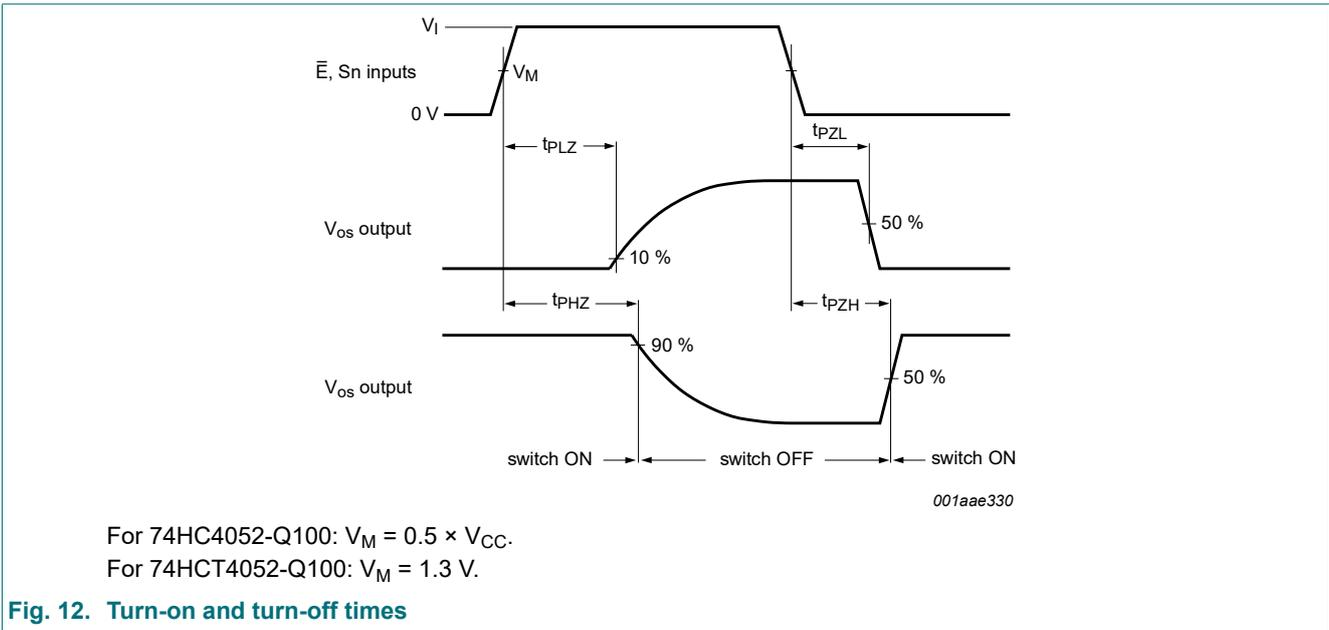
Fig. 12. Turn-on and turn-off times
