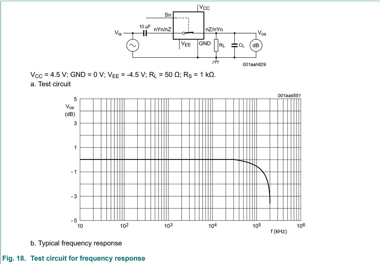
Fig. 18. Test circuit for frequency response
