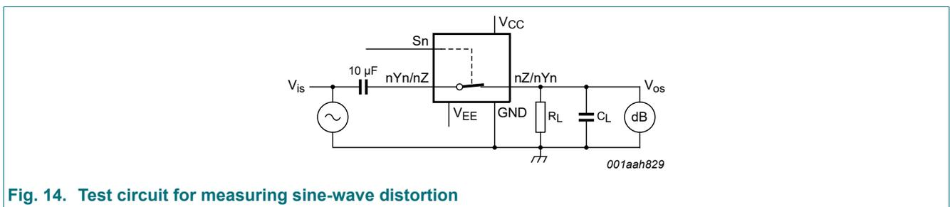
**Fig. 14. Test circuit for measuring sine-wave distortion**
