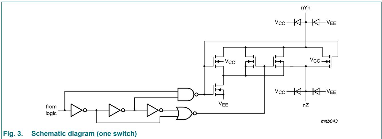
Fig. 3. Schematic diagram (one switch)
