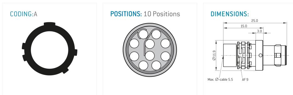
The pin layout corresponds to the view on the termination area
