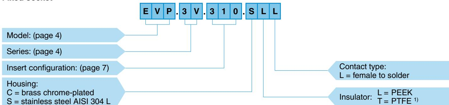
**EVP.3V.310.SLL** = fixed socket, nut fixing, 3V series, multipole type with 10 contacts, outer shell in stainless steel, PEEK insulator, female solder contacts.
