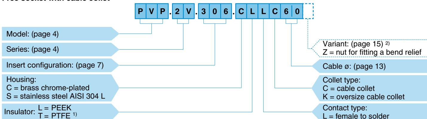
**PVP.2V.306.CLLC60** = free socket with cable collet, 2V series, multipole type with 6 contacts, outer shell in chrome-plated brass, PEEK insulator, female solder contacts, C type collet for 6 mm diameter cable.
