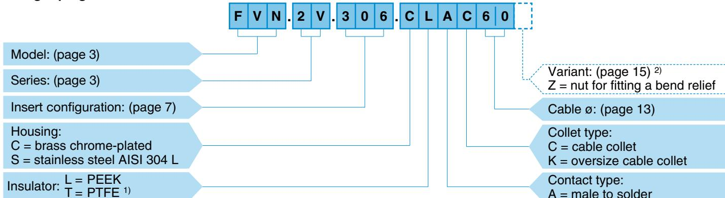
**FVN.2V.306.CLAC60** = straight plug with cable collet, 2V series, multipole type with 6 contacts, outer shell in chrome-plated brass, PEEK insulator, male solder contacts, C type collet for 6 mm diameter cable.
