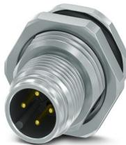
Sensor/actuator panel-mount connector, 4-pos., M12 push-pull, rear/screw mounting with M16 thread, with 0.50 m litz wire, 4x 0.34 mm<sup>2</sup>
