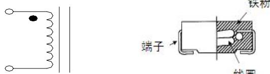
绕线结构表 Winding Structure Diagram
