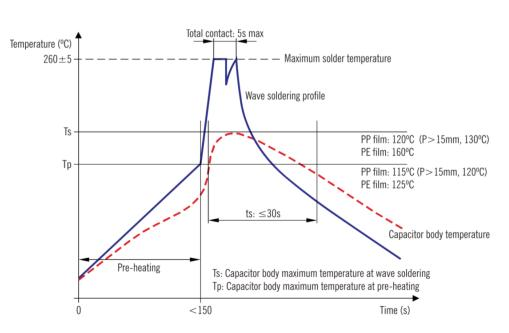
preheating temperature, preheating time, soldering temperature, soldering time, other heat sources influence and so on.
