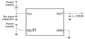
\* Disable current test should be  $OE = \overline{GND}$ . Stand-by current test should be  $\overline{ST} = \overline{GND}$ .
