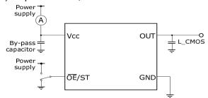
\* Disable current test should be  $\overline{OE} = V_{CC}$ . Stand-by current test should be  $ST = V_{CC}$ .
