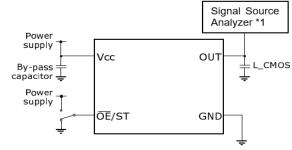
\*1 Signal Source Analyzer: Keysight: E5052B, Minimum frequency = 10 MHz
