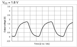
fo = 150 MHz, L\_CMOS = 15 pF, T\_use = +25 °C, Rise/Fall time: A (Default) or B (Faster)
