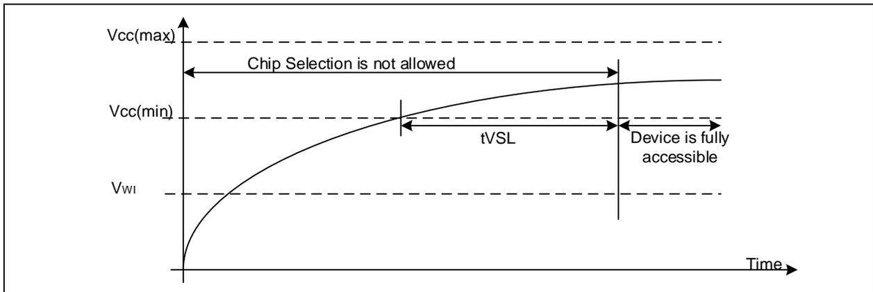
Table 9. Power-Up Timing and Write Inhibit Threshold
