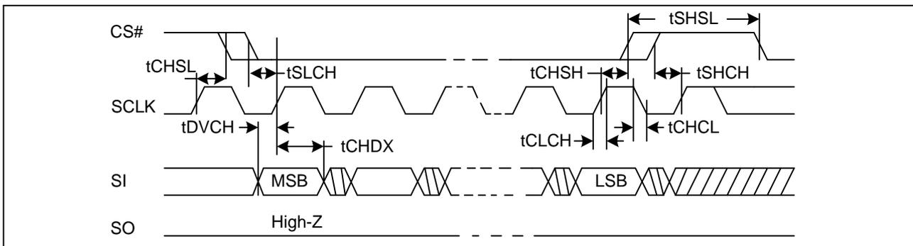
**Figure 41. Output Timing**
