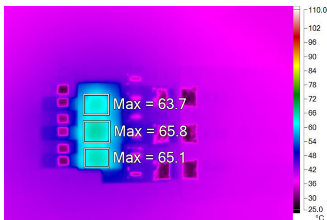
Figure 5. Thermal Image, Full Load with Three Channels in Parallel (1.3V IN , 1V OUT , 9A) without Fan, T A = 25°C
