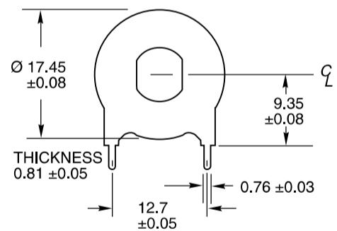
For printed circuit styles. Mounting bushing provides additional support for the front end of the switch. Order separately by appropriate part number. Rotary switch discount applies.
