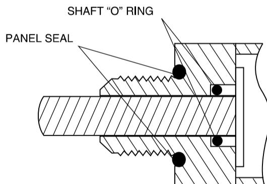
The shaft is sealed by an O-ring inside the bushing. The panel is sealed by an O-ring at the base of the bushing.
