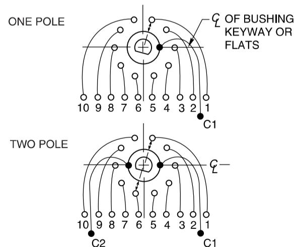
**SERIES 71: PC Board Pattern** in inches (and millimeters)
