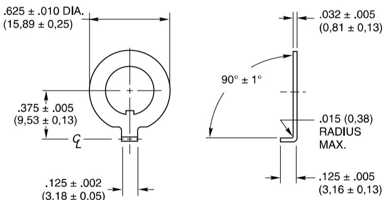
**4mm Diameter Shaft Switches****Non-Turn Washer**
