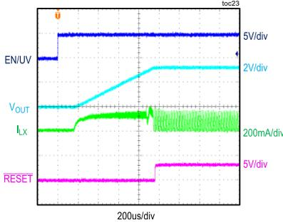
CONDITIONS: 3.3V OUTPUT, 66Ω LOAD,  $f_{SW} = 70kHz$
