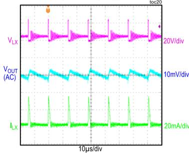
CONDITIONS: 5V OUTPUT, 1mA LOAD,  $f_{SW} = 70kHz$
