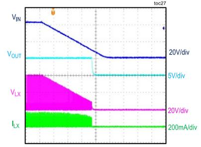
CONDITIONS: 5V OUTPUT, 100Ω LOAD,  $f_{SW} = 70kHz$
