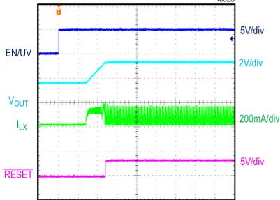
CONDITIONS: 3.3V OUTPUT, 66Ω LOAD,  $f_{SW} = 70kHz$
