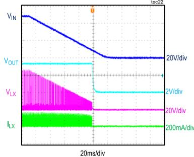
CONDITIONS: 3.3V OUTPUT, 66Ω LOAD,  $f_{SW} = 70kHz$
