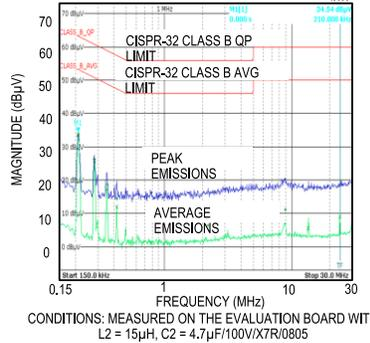
CONDITIONS: MEASURED ON THE EVALUATION BOARD WITH  $L2 = 15\mu H$ ,  $C2 = 4.7\mu F/100V/X7R/0805$
