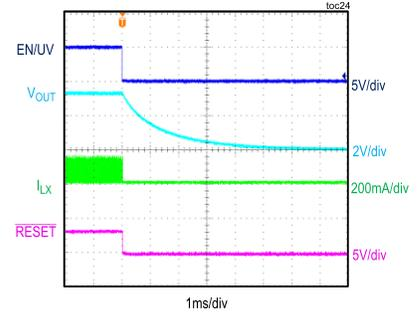
CONDITIONS: 3.3V OUTPUT, 66Ω LOAD,  $f_{SW} = 70kHz$
