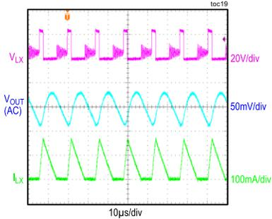
CONDITIONS: 5V OUTPUT, 50mA LOAD,  $f_{SW} = 70kHz$
