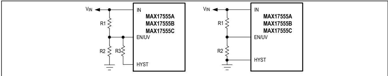
Figure 1. Setting the Input Undervoltage Level with and without Hysteresis
