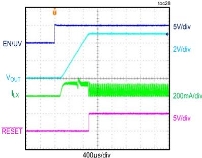
CONDITIONS: 5V OUTPUT, 100Ω LOAD,  $f_{SW} = 70kHz$
