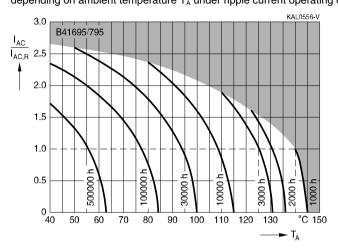
$\begin{tabular}{ll} \textbf{Useful life}^{1)} \\ \textbf{depending on case temperature $T_{C}$ under ripple current operating conditions at $V_{R}$} \\ \end{tabular}$
