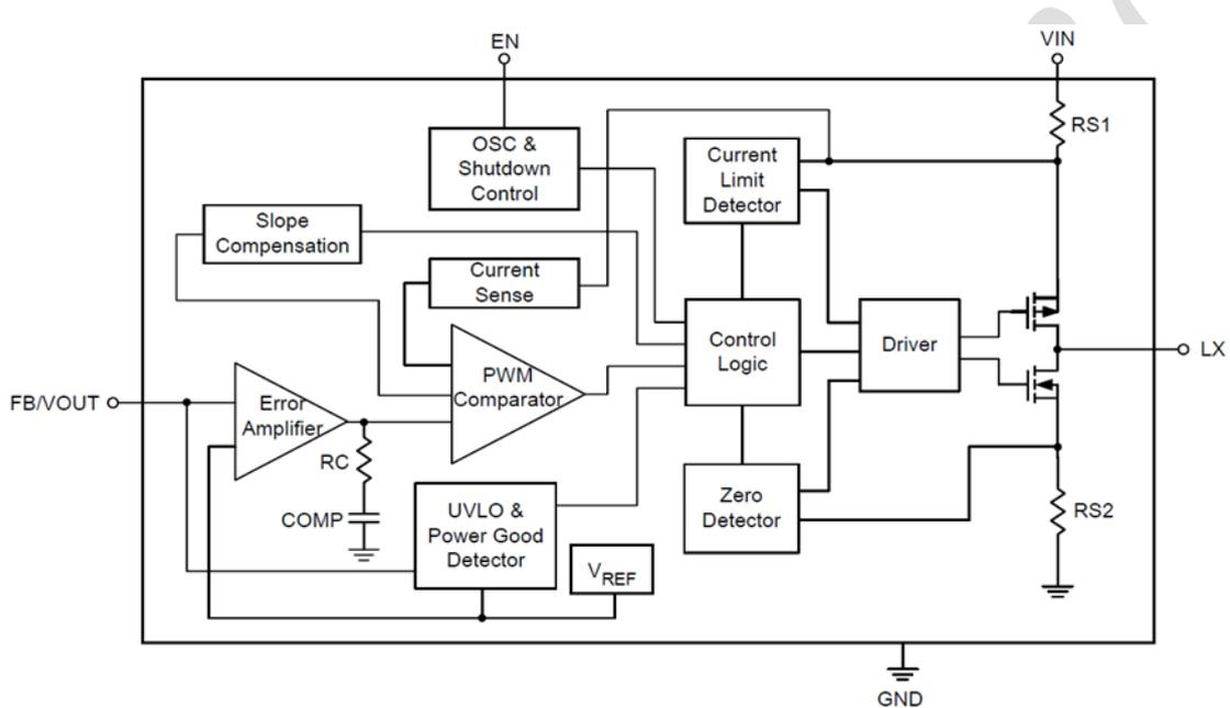
Figure 3. STI3408B Block Diagram
