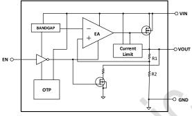
Figure 3. TMI6050 adjustable function block
