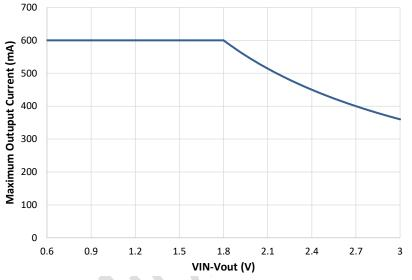
Figure 7. curve of maximum output current vs. VIN-VOUT
