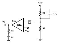
Figure 5. Application Circuits of Feedforward Capacitor  $C_{\mbox{\scriptsize FB}}$
