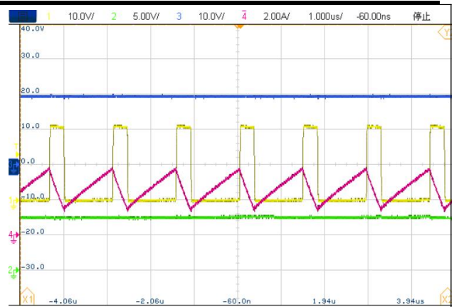
Fig. 9 Steady state waveform, Iout = 0.5A
