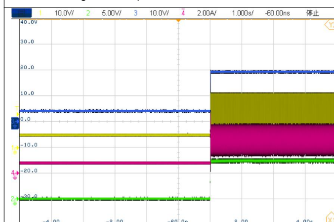
Fig. 4 Startup waveform VIN, Iout = 0.5A
