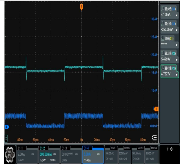
Ch2: Vout Ch4: Iout Vin=60V Vout=12V
