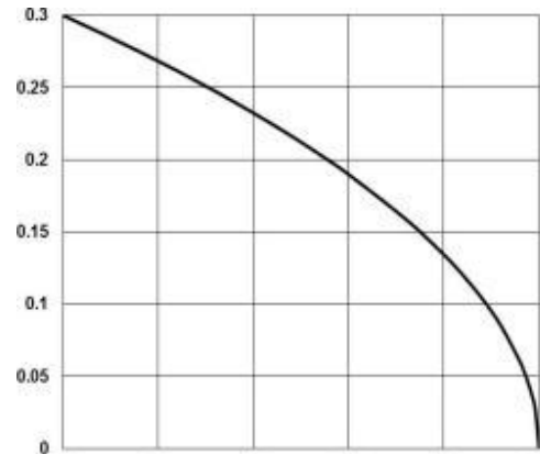
Fig. 2 Continuous Drain Current vs. T_J
