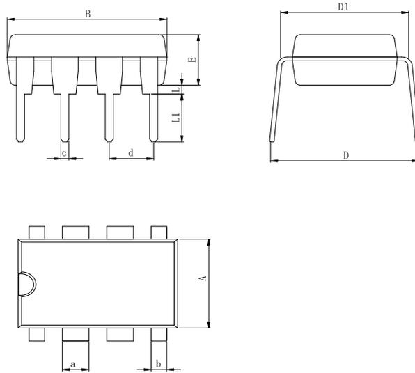
Dimensions In Millimeters(DIP-8)
