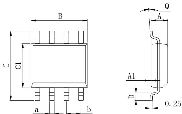
Dimensions In Millimeters(SOP-8)
