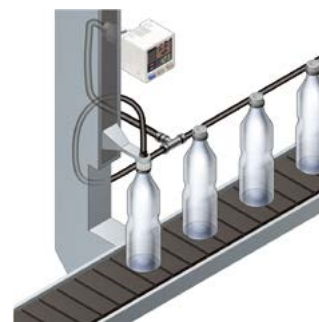
Air-leak test for PET bottles
