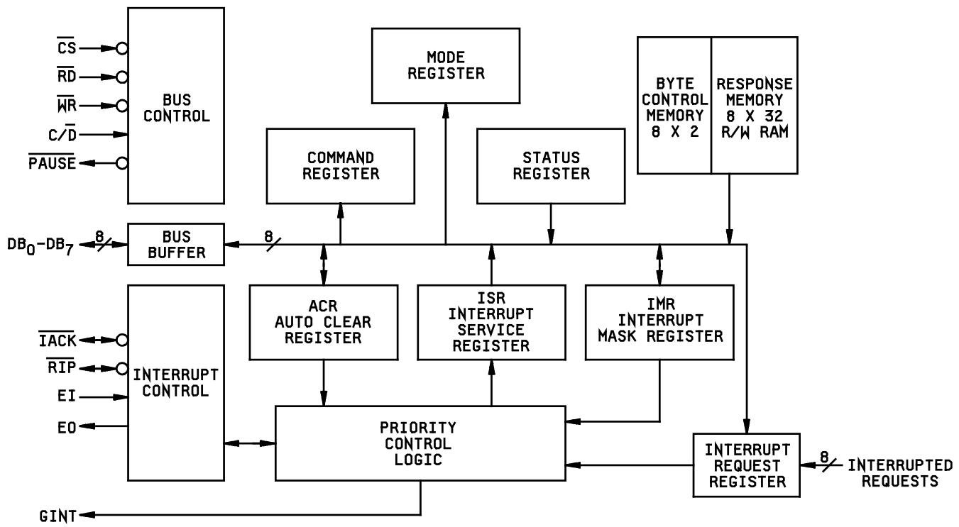
FIGURE 3. Block diagram.
