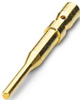
Crimp contact, Pin, turned, contact diameter: 1.5 mm, crimp range: 0.5 mm<sup>2</sup> ... 1 mm<sup>2</sup>,
