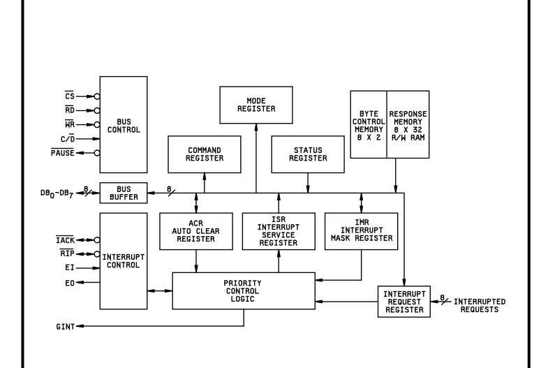
FIGURE 3. Block diagram.
