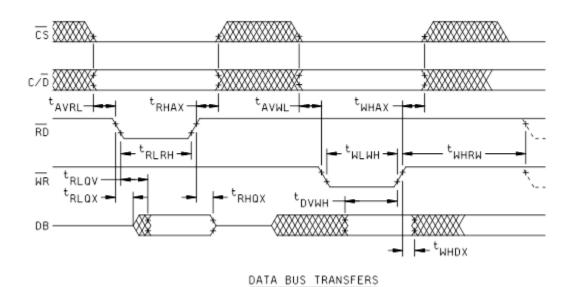
FIGURE 4. Switching waveforms.
