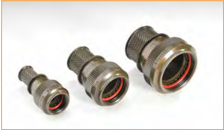
BT Series backshells terminate the shield with a stainless steel band strap. Additional strain relief can be obtained with a heat-shrink boot.
