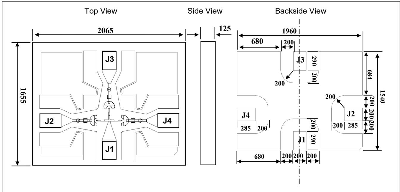
9. Bottom view shows the back metal foot print and mounting pads.
