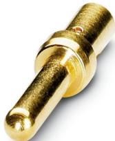
Crimp contact, Pin, turned, Single contact, contact diameter: 1 mm, crimp range: 0.14 mm<sup>2</sup> ... 0.56 mm<sup>2</sup>, Contact release tool not necessary for the 12- and 17-pos. crimp versions of the M23-PRO series, Alternative product in accordance with RoHS II without Exemption 6c (Pb < 0.1 %) item no.: 1240882
