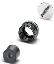
Cable clamp type cage and shield adapter, shielded: yes, litz wire bundle diameter: 4.6 mm, cable diameter range: 6.5 mm ... 7.5 mm, series: NC, RC
