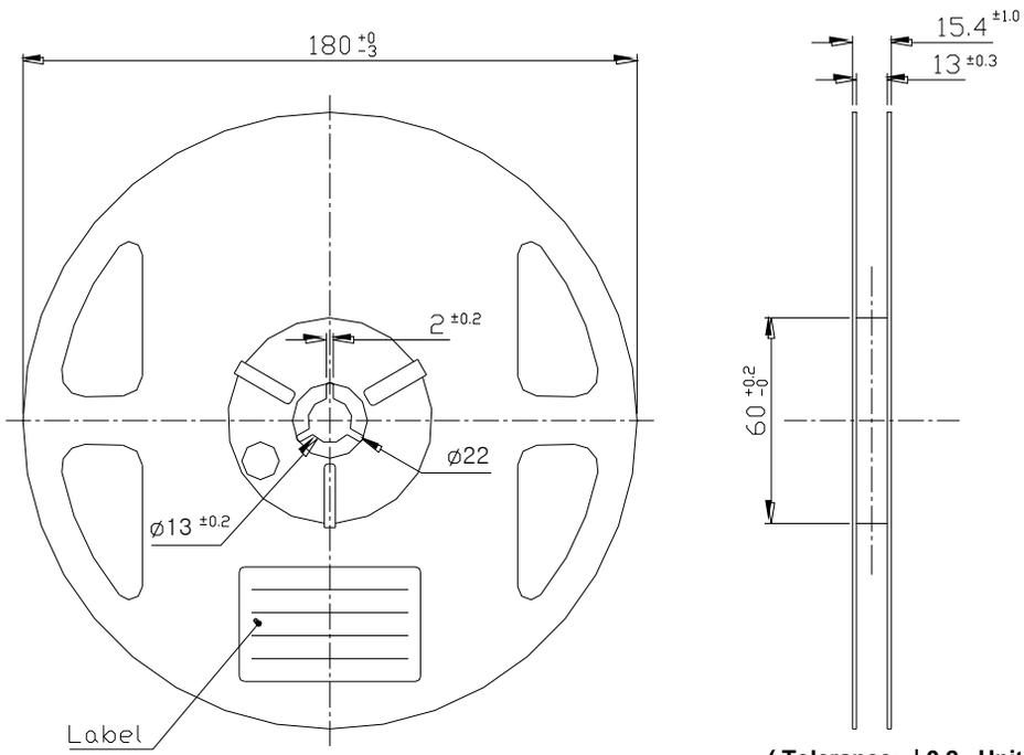
(Tolerance:  $\pm 0.2$ , Unit: mm)
