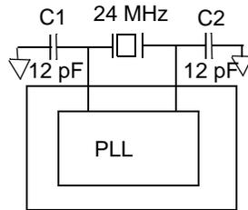
12 pF capacitor values assumes a trace capacitance of 3 pF per side on a four-layer FR4 PCA
