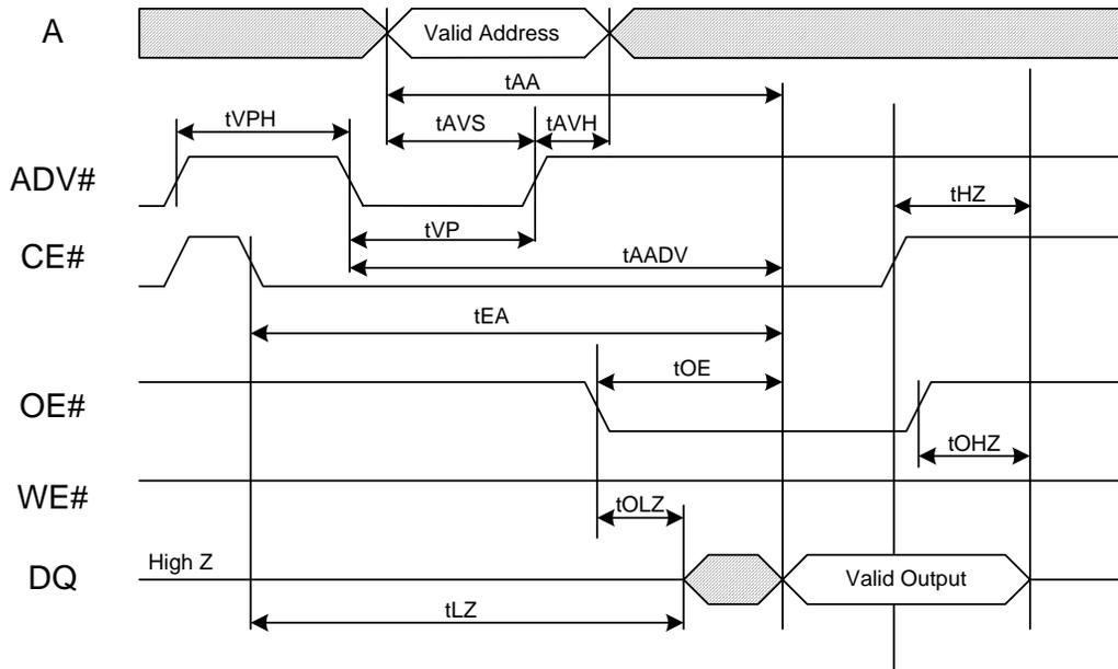
Figure 5. Asynchronous Back-to-Back Read Timing
