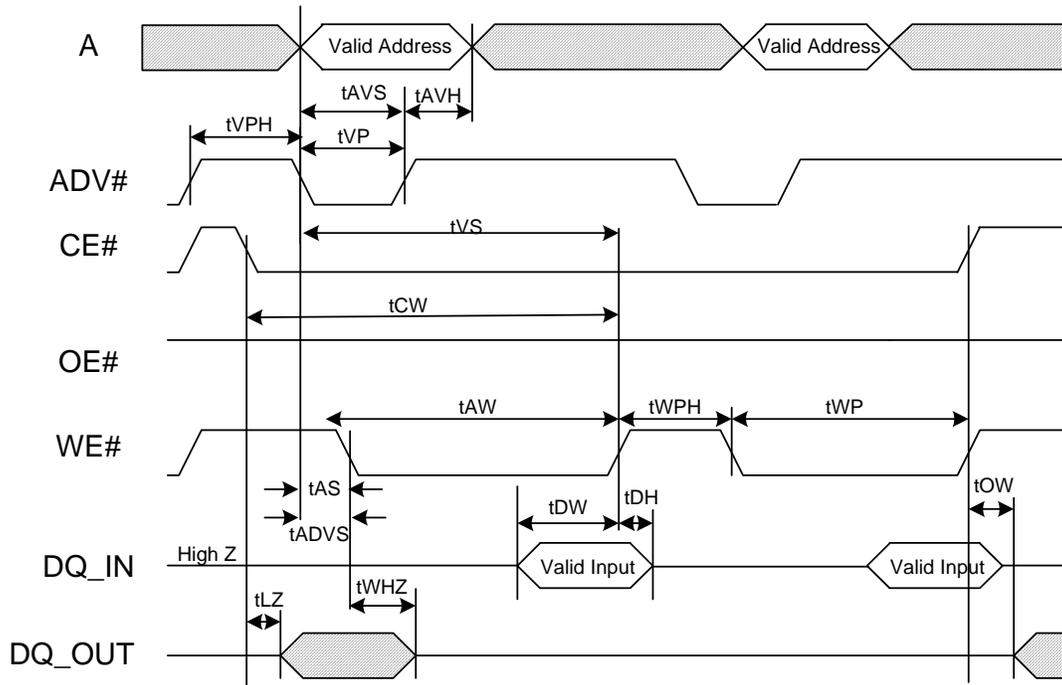
Figure 7. Asynchronous Read to Write Timing
