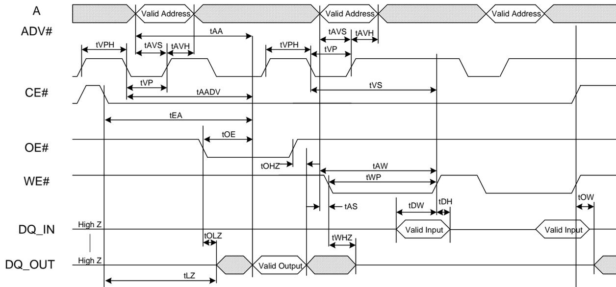
Figure 8. Asynchronous Write to Read Timing
