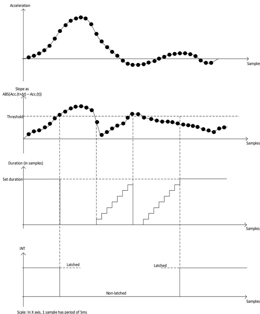
Register FEATURES\_IN.no\_motion.settings\_2.duration defines the number of consecutive data points for which the slope of enabled axis must be smaller than the threshold for an interrupt to be asserted.
