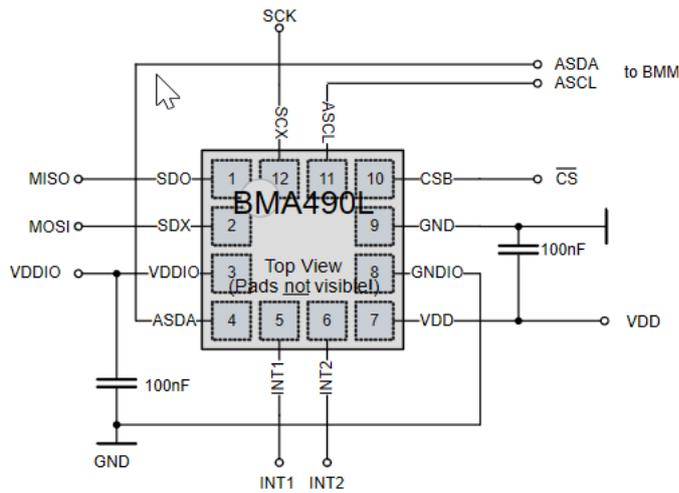
It is recommended to use 100nF decoupling capacitors at pin 3 (VDDIO) and pin 7 (VDD).
