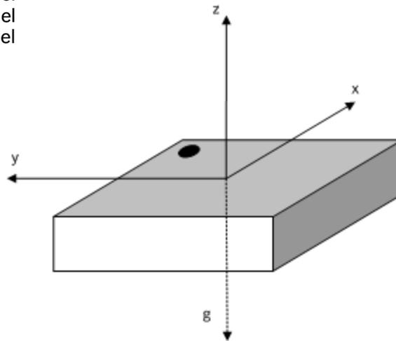
The following table lists all corresponding output signals on X, Y, and Z while the sensor is at rest or at uniform motion in a gravity field under assumption of a  $\pm 4g$  range setting, a 16 bit resolution, and a top down gravity vector as shown above.
