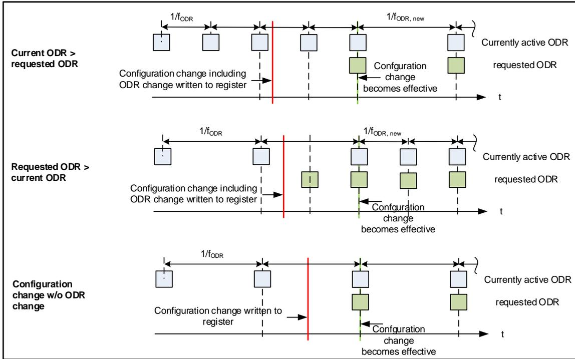
Due to filter settling, some invalid samples can be suppressed in addition after a configuration change.
