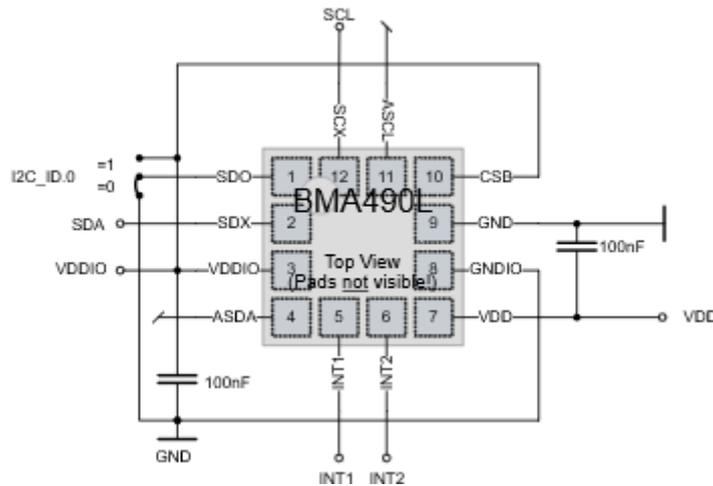
It is recommended to use 100nF decoupling capacitors at pin 3 (VDDIO) and pin 7 (VDD). SDA and SCL should be connected to  $V_{DDIO}$  externally via pull-up resistors so that they are pulled high when the bus is free.
