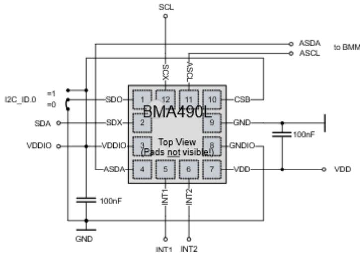
It is recommended to use 100nF decoupling capacitors at pin 3 (VDDIO) and pin 7 (VDD). SDA and SCL should be connected to  $V_{DDIO}$  externally via pull-up resistors so that they are pulled high when the bus is free.
