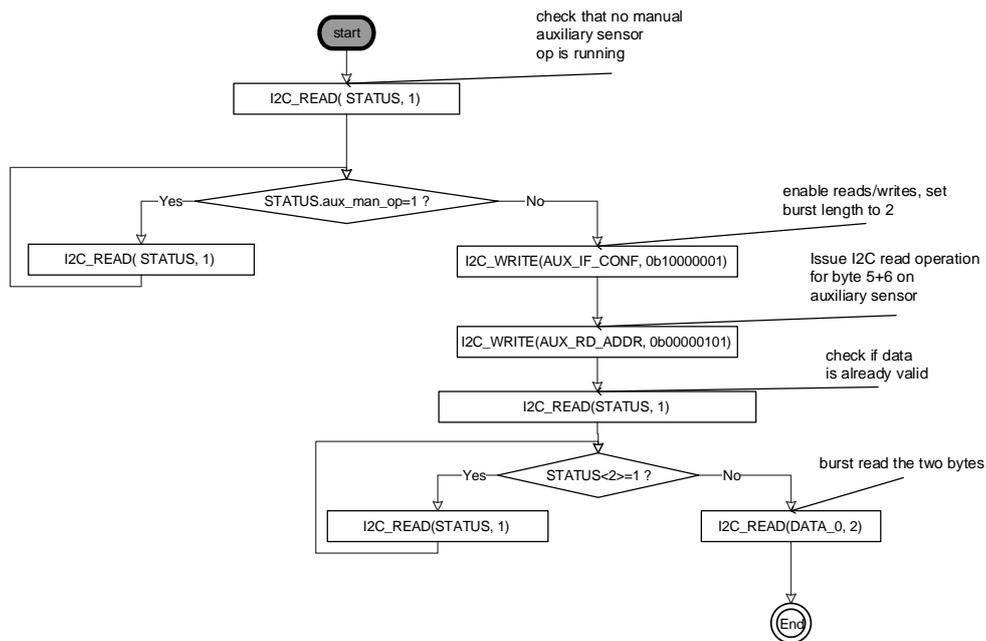
Example: Write 0xEF into register 3 of auxiliary sensor
