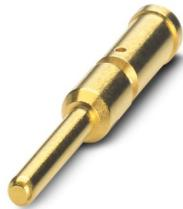
Crimp contact, Pin, turned, contact diameter: 2 mm, crimp range: 0.25 mm<sup>2</sup> ... 1 mm<sup>2</sup>, Alternative product in accordance with RoHS II without Exemption 6c (Pb < 0.1 %) item no.: 1238179
