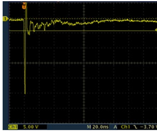
SP1112 IEC 61000 -4-2 -8 kV Contact ESD Clamping Voltage
