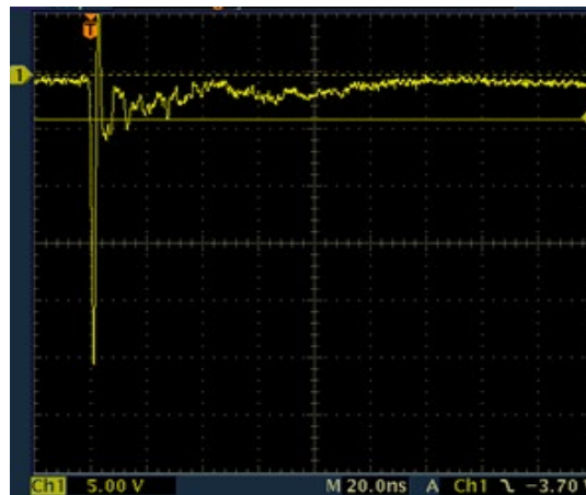
SP1112 IEC 61000 -4-2 -8 kV Contact ESD Clamping Voltage
