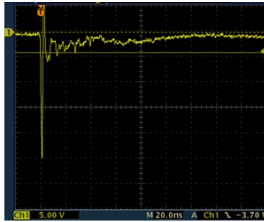
SP1105S IEC 61000 -4-2 -8 kV Contact ESD Clamping Voltage
